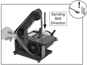
Figure 14. Replacing sanding belt.
